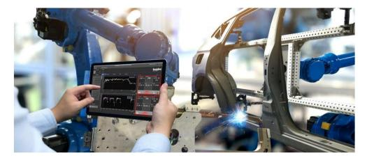
Leadec's welD.One software solution ensures an optimal representation of current welding data and permanent quality control in the production.
